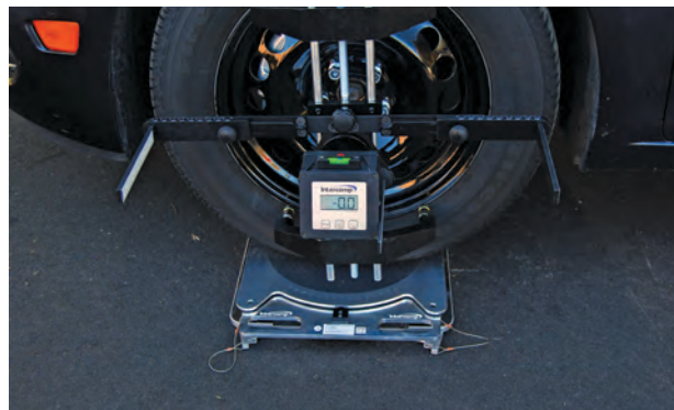
The AS2000™ alignment system utilizes laser alignment heads, mounted on each wheel, to ensure all four wheels are aligned to manufacturer specifications.
